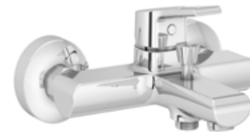
Single lever bath and shower mixer DN 15 Ceramic cartridge -K35 without shower set PCA aerator M 24 X 1 flow class CB automatic diverter shower to bathtub shower outlet G 1/2" protected against back flow S-unions 1/2 x 3/4 inch European standard - EN 817
