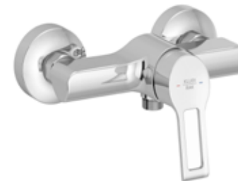
Single lever shower mixer DN 15 Ceramic cartridge - K35 flow class B shower outlet G 1/2" protected against back flow S-unions 1/2 x 3/4 inch European standard - EN 817
