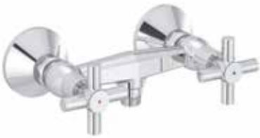
RAK34010 Dual controlled shower mixer DN 15 ceramic head part 90 ,Right & Left flow class B shower connection 1/2 inch protected against back flow S-unions 1/2 inch x 3/4 inch in accordance to EN 200
